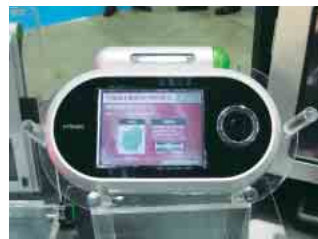
PDA concept model with electrode imbedded. The green tube is a cartridge containing methanol solution.
