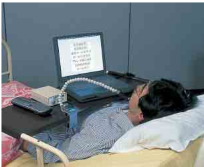
This device assists amyotrophic lateral sclerosis (ALS) patients in writing and using PCs.
