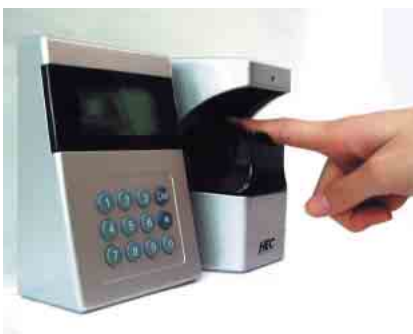
This system realizes higher security by using authentication method to read finger vein patterns.
