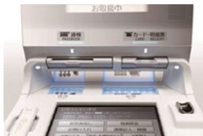
An arched guide frame leads hands naturally toward the slots.
