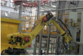
Loading an elevator hatch for coating.
