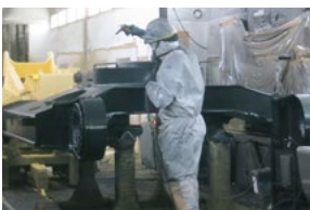
Coating the frame of a hydraulic excavator.
