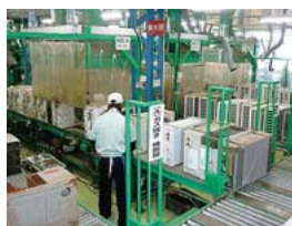
Air conditioner recycling
