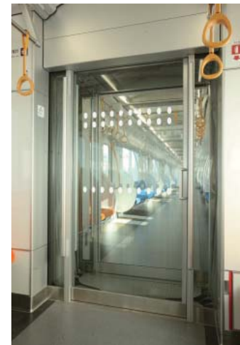
SEIBU Railway Series 30000 commuter trains feature large glass doors at the ends of train cars
