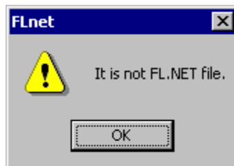
Figure 5-51 The Error Message Dialog Box Displayed in the Event of a Non-Existent or Invalid FL.NET Setup Info File Specified
