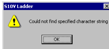
Figure 4-25 Search Result Message Dialog Box Displayed When Not Finding Matching Ladder Symbol
