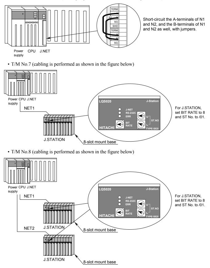
• T/M No.5 and T/M No.6 (cabling is performed as shown in the figure below)
