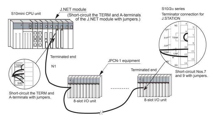
• Connection when the J.NET module is not used at an end of N1
