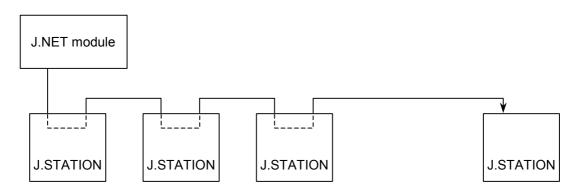
J.STATIONs are mounted on an I/O unit to constitute a remote I/O unit.
