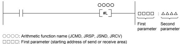
$\triangle \triangle \triangle \triangle$ : Second parameter (number of send/receive area bytes)
