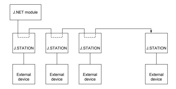
• When the J.NET module is connected to J.STATIONs (data transmitted)
