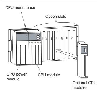
CPU extension mount base: HSC-1080 PS slot: Slot into which the CPU power supply (LVQ000) is inserted. CPU slot: Slot into which a CPU module (LQP000, LQP010) is inserted. Slot 0 to slot 7: Slots into which CPU optional modules or I/O modules are inserted.
