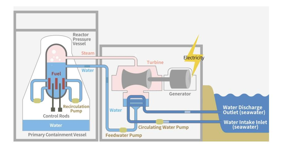
Nuclear power generation produces electricity in a similar way to thermal power generation. In both cases, boil water and convert it into steam, using that steam to turn large impellers known as turbines to operate a generator and produce electricity. While thermal power generates heat by burning coal, oil and natural gas, nuclear power generation uses the heat generated by the fission of uranium fuel inside a reactor.
