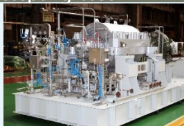
Process compressor for ammonia plants
