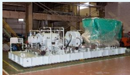
CO 2 compressor for CCS
