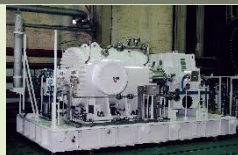
Compressor for pipelines
