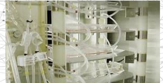
Automated cell mass culture for iPS cells* Applied to a clinical trial for Parkinson's disease (Manufacturer: SDP, Clinical: Kyoto University) (Announced in January 2021)
