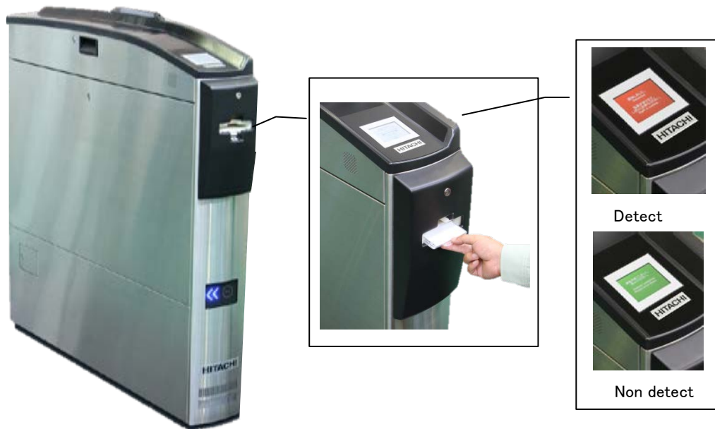
Walk-through type explosives trace detection system
