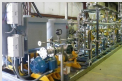
Contaminated water treatment system (Example)
